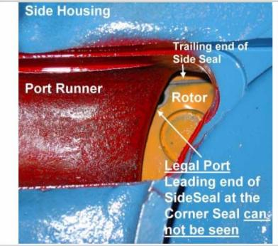
Cut-away view of what the Tech Inspectors will be seeing with borescope or mirror and penlight.
