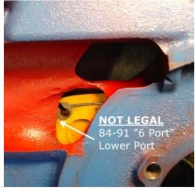
Cut-away of intake port showing port wall moved beyond the scribed arc. Image is actual 84-91 13B "6-Port" Iower intake port, but also applies to all "4-Port" engines.
