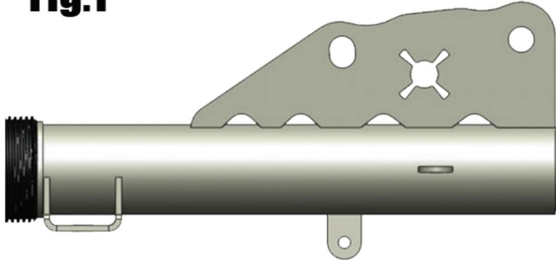
Figure 2: SMG Strut Housing with Camber Slug Installed.
