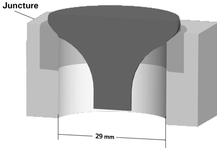
10. Replacement of intake and exhaust valve seats is allowed for the purpose of repair only. Valve Seats may not be moved from their original position. Welding is allowed to facilitate repair and installation of replacement seats. The original size and shape of the combustion chamber must be maintained. Installed seats may neither be proud or recessed of the combustion chamber surface.
