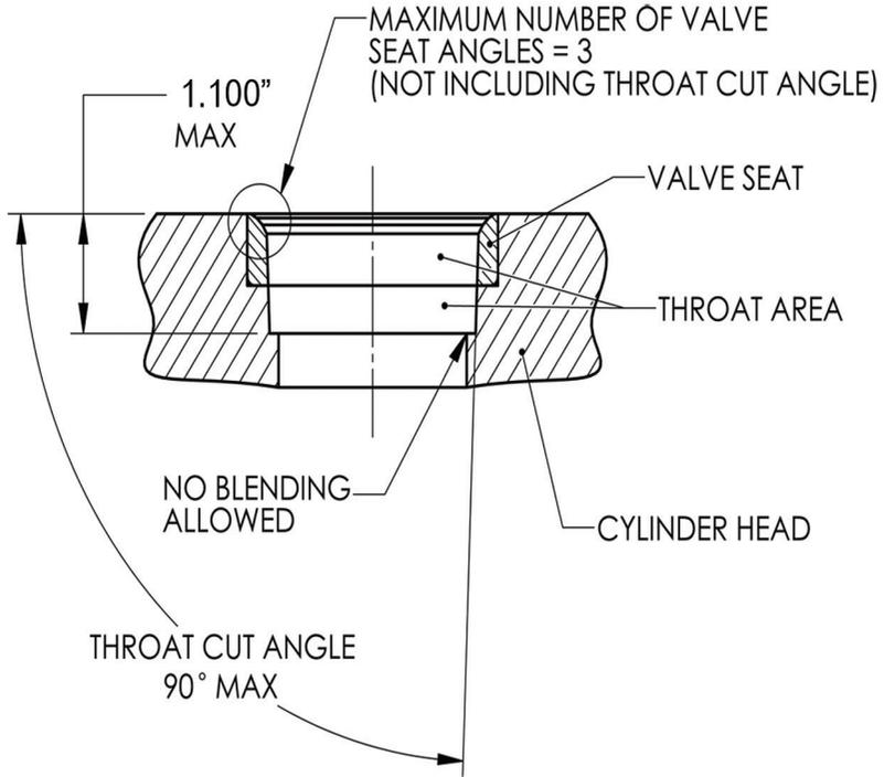
**Figure 2 Aluminum Cylinder Head Repair Zone**
