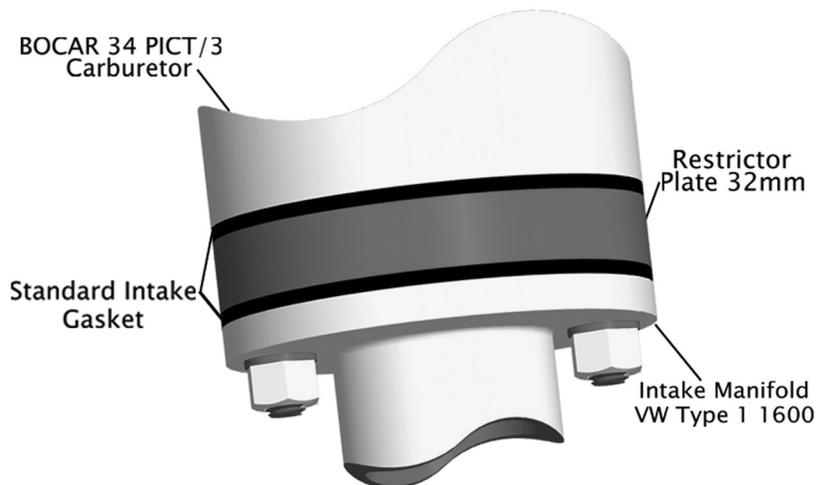
4. (1) Standard VW (or direct replacement) carburetor gasket
